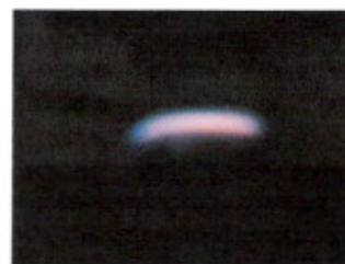
Fig. 6 Opposed-flow flame, flow speed = 25 cm/s.
